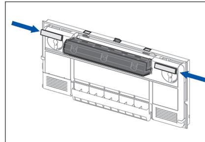
5. Slide the two new filters fully into the filter housing so that they do not project.
