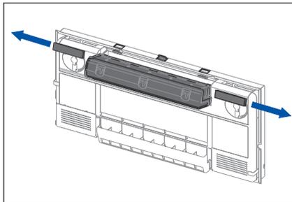
4. Slide the two contaminated filters to the sides out of the filter housing.
