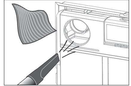
12. Remove any dirt from both channels with a vacuum cleaner or a soft cloth (do not use water).
