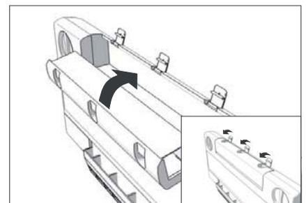
6. Tilt the filter housing upwards and secure with the three clips.
