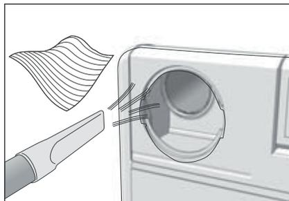
5. Remove any dirt from both channels with a vacuum cleaner or a soft cloth (do not use water).
