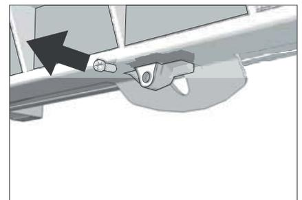
3. Loosen the two screws under the filter cover.
